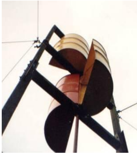
Figure 13: VAWT (Savonius type) for electricity generation
