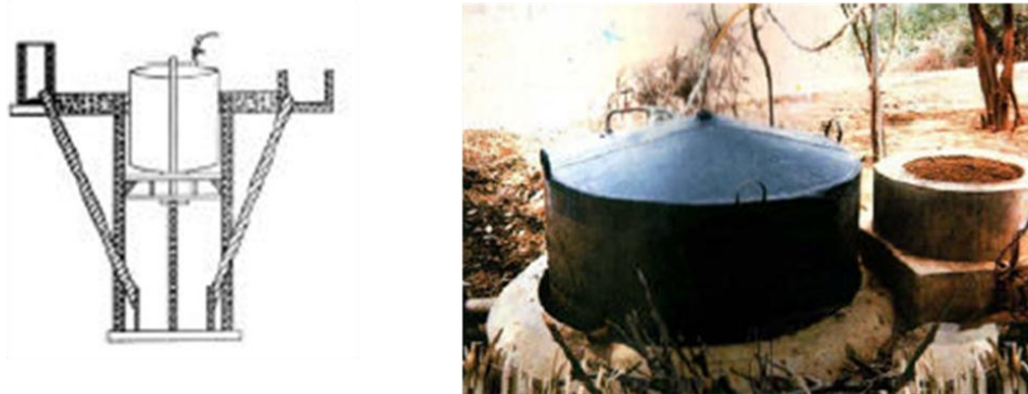
Fig: Indian floating drum gas holder
