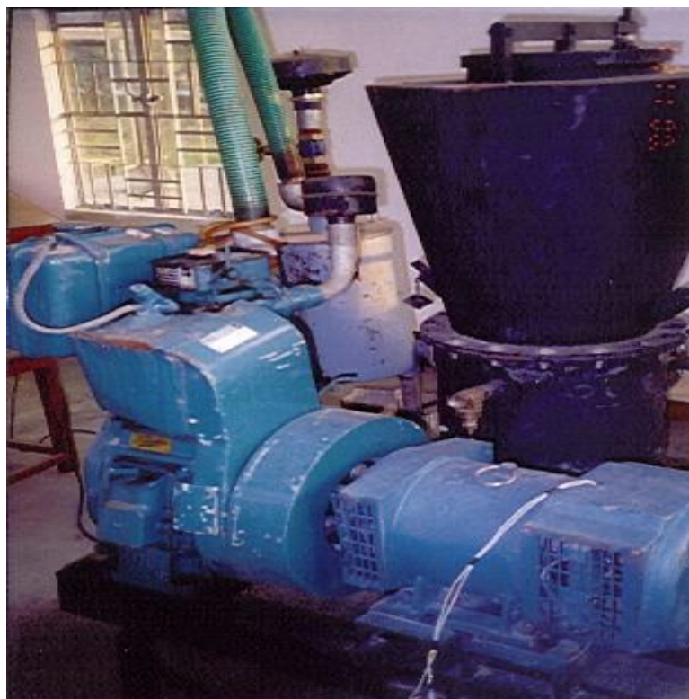
5 kw Biomass Gasifier Unit
