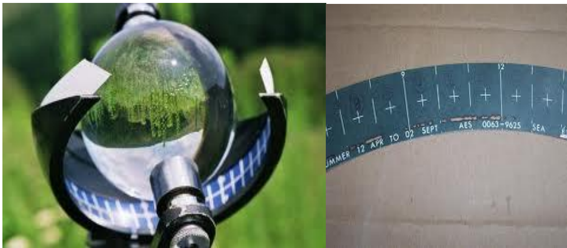
Fig. 9. Photograph of Sunshine duration recorder and the calibrated strip
