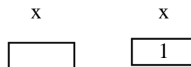
Figure 2. (a) A variable x is declared, but not initialized blank (b) a variable x is initialized with the value 1.
