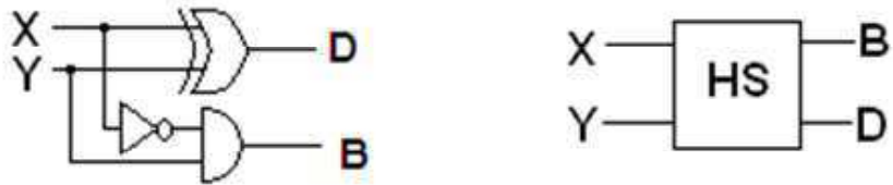
Figure 2.3: The Half-Subtractor circuit and symbol
