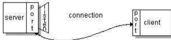
Fig. 5.2 Client socket and port number
