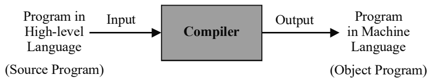
Fig. 1.35 Translation Process using a Compiler
