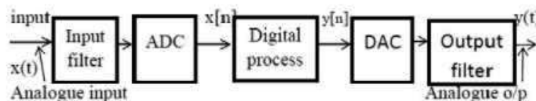
Fig. 5.4 A Simplified Block Diagram illustrating the Operation of a Real-Time Digital Filter with Analogue Input and Output Signals
