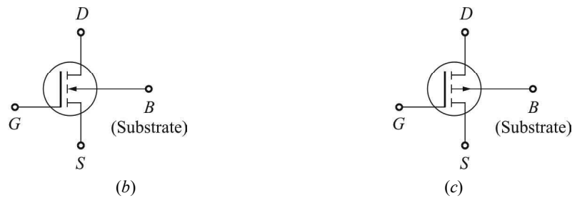
Fig. 5.9 (a) Structure of N -channel enhancement MOSFET, (b) and (c) Circuit symbols of N -channel and P -channel enhancement MOSFETs
