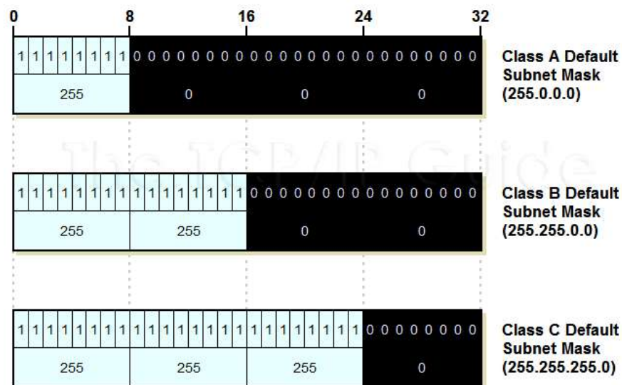
Fig. 4.47 Default Subnet Masks for Class A, Class B and Class C Networks
