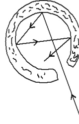
Fig. 5.6 Absorption of radiations in a blackbody
