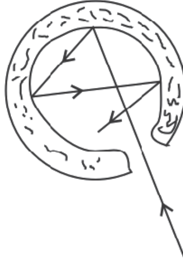
Fig. 2.10 Absorption of radiations in a blackbody
