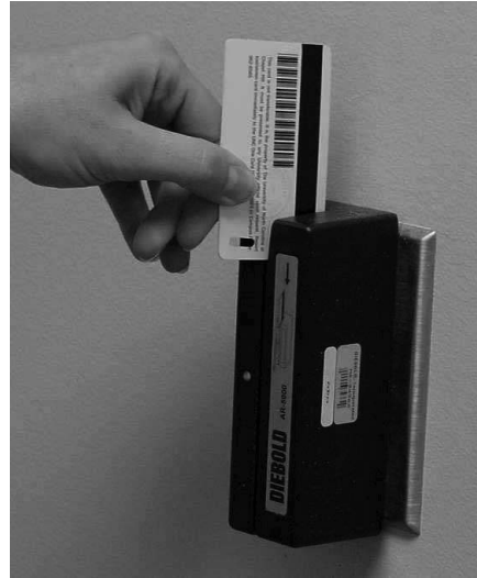
Fig. 1.29 An Access Card Security System
